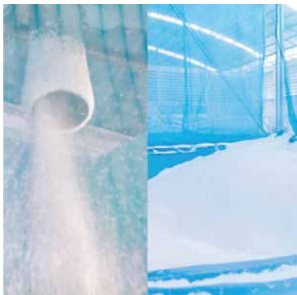
EPS in Silo
